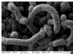
Positive electrode-polypyrrole deposited by cyclic voltammetry on CNTs
